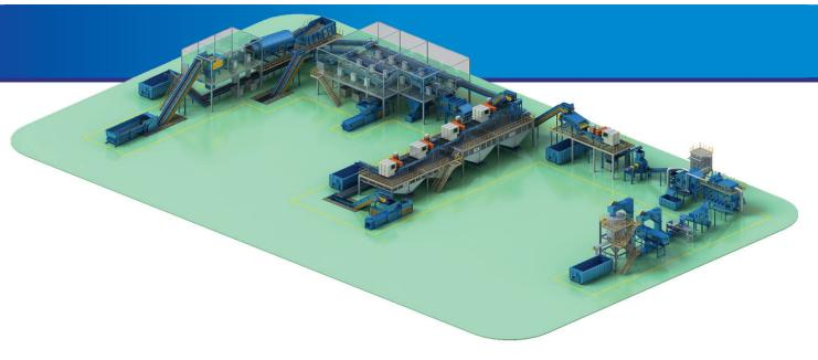
Bag opener + Dynamic separator + trommel + Ballistic + Magnetic + Eddy-current + NIR sorter + Air separator + Dryer + Extruder
